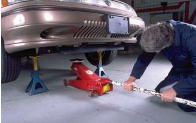
Figure1- 9 whenever you have raised a vehicle with a floor jack, the vehicle should be supported with jack stands.
