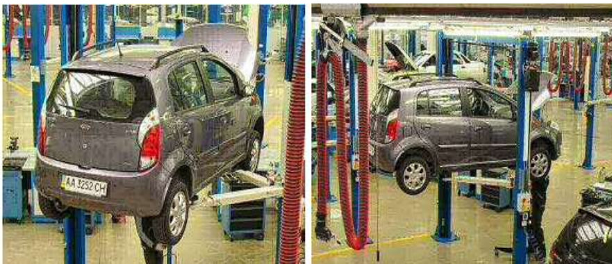
Figure1- 17 Hydraulic lift with hoist arms that raise the vehicle on its lifting points. The lift consists of two vertical blue beams and four white hoist arms. Two white hoist arms on the other side of the vehicle are not seen in the pictures.
