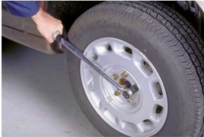
Figure1- 3 Wheel lugs should be tightened to the specified torque.
