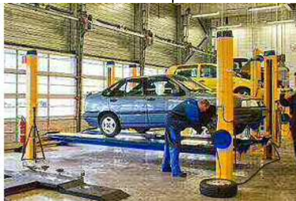
Figure1- 18; Another hydraulic lift that raises the car on its tires
