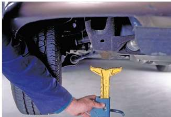
Figure1- 14 Jack stands should be used to support the vehicle after it has been raised by a jack.
