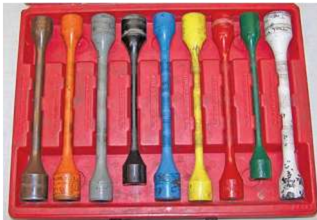
Figure1- 4 Torque sticks are color coded to indicate their torque setting.
