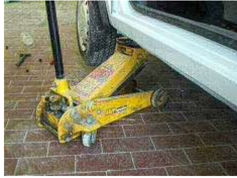
Figure1- 16 Hydraulic jack with hand-pump mechanism
